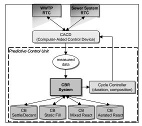
Figure 6: Principle of the predictive SBR controller.
