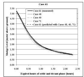
Figure 8: Good prediction of the sludge settling curve.
