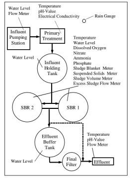
Figure 5: Scheme of WWTP Messel
