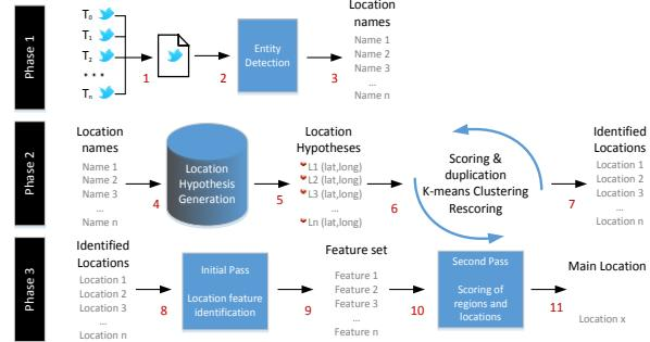
**Fig. 2.** Three phases of the Content-based Geo-location Clustering and Detection Algorithm
