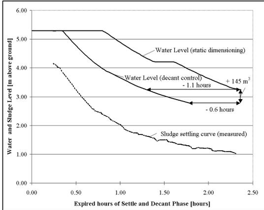
Figure 7: Potential for optimisation of settle and decant phase.
