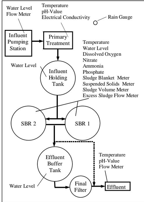
Figure 5: Scheme of WWTP Messel
