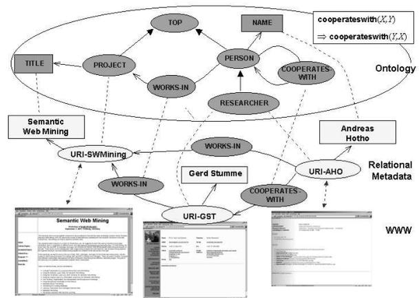
Fig. 2. The relation between the WWW, relational metadata, and ontologies.
