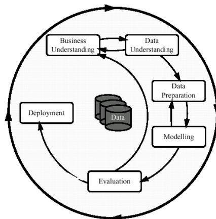
Figure 2: Phases of the CRISP-DM Reference Model
