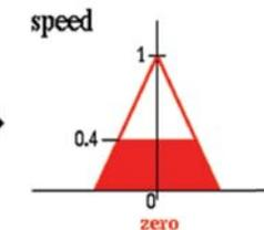
Since the two parts of the condition of our rule are connected by an AND we calculate  $\min(0.75, 0.4) = 0.4$  and cut the fuzzy set "zero" of the variable "speed" at this level (according to our rule).
