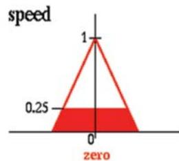
If angle is positive low and angular velocity is negative low then speed is zero
