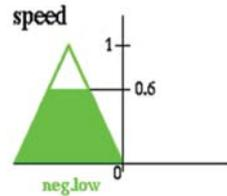
If angle is zero and angular velocity is negative low then speed is zero
