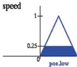
If angle is positive low and angular velocity is zero then speed is positive low
