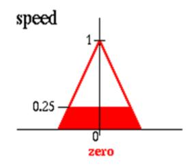
If angle is positive low and angular velocity is negative low then speed is zero
