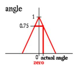
If angle is zero and angular velocity is zero then speed is zero
