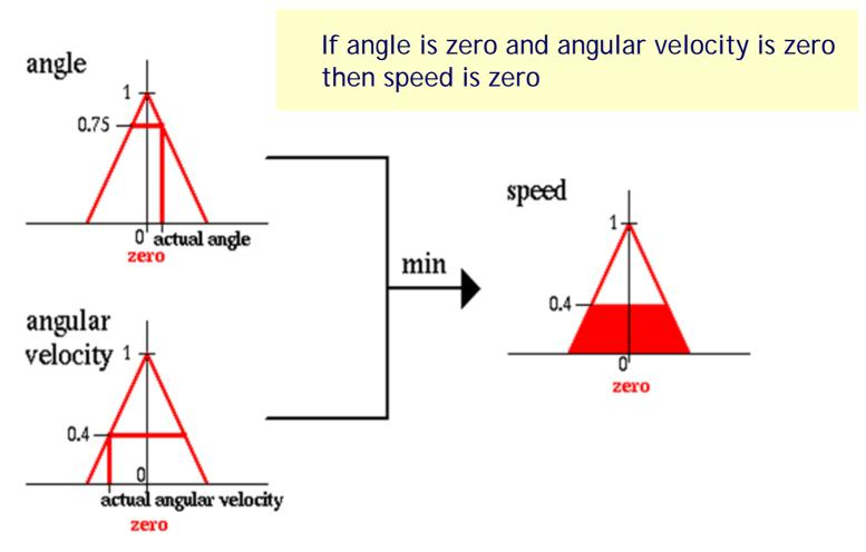
Since the two parts of the condition of our rule are connected by an AND we calculate min(0.75,0.4) = 0.4 and cut the fuzzy set "zero" of the variable "speed" at this level (according to our rule).
