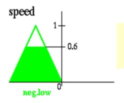
If angle is zero and angular velocity is negative low then speed is zero
