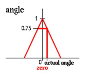
If angle is zero and angular velocity is zero then speed is zero
