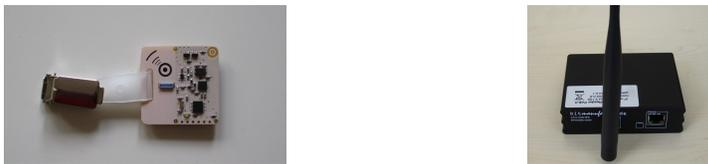
**Fig. 1.** Proximity tag (left) and RFID reader (right)
